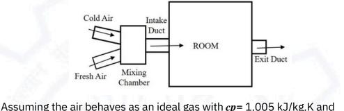
Assuming the air behaves as an ideal gas with *cp*= 1.005 kJ/kg.K and *R*= 0.287 kJ/kg.K, the rate of heat gain by the air from the room is \_\_\_\_\_\_ kW(*round off to two decimal places*).
