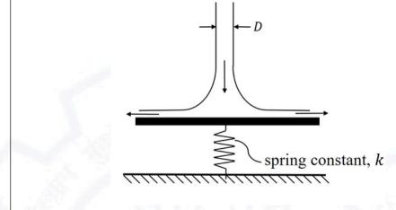
If the spring shows a steady deflection of 1 cm upon impingement of jet, then the velocity of the incoming jet is \_\_\_\_\_ m/so(und off to one decimal place).
